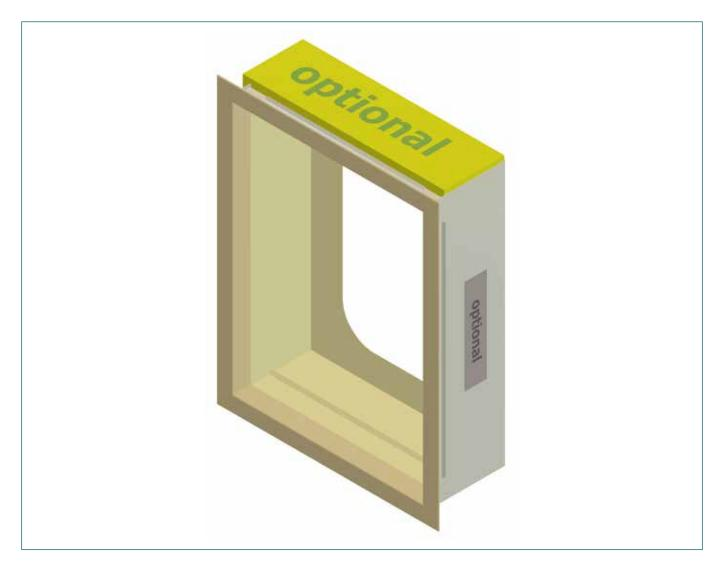
The window box provides the connection between the hull and the accommodation system and consists of two elements, the basic body with a prefabricated window cut-out and the sliding frame, that is used to compensate for tolerances. According to customer specifications the basic body can optionally be produced insulation-padded or with noise suppression plates on the outside and a condensation trap on the bottom line.
