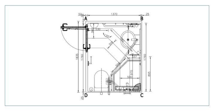
The wet unit Type Passenger cabin layout is for passenger cabins on board of every types of ships and maritime facilities. It consists of a toilet, a shower with a glass wall and door as well as a washbasin. A large variety of equipment is available. The wet units meet all individual needs, are manufactured according to the highest quality standards and comply with the most recent safety regulations.
