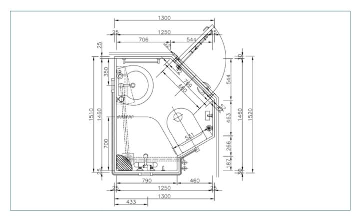
The wet unit Type Crew cabin layout is for crew cabins on board of every types of ships and maritime facilities. It consists of a toilet, a shower with a curtain and washbasin. A large variety of equipment is available. The wet units meet all individual needs, are manufactured according to the highest quality standards and comply with the most recent safety regulations.
